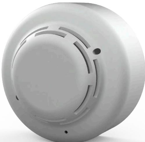
Upon activation, the detector remains in the alarm state until a reset command is issued from the fire alarm control panel. Dual LED indicators provide visual feedback—flashing periodically in standby mode and remaining steadily illuminated during alarm condition.
