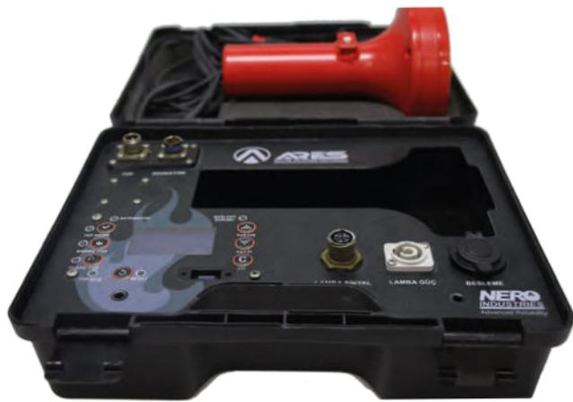
The test kit is designed and produced to measure whether there are any faults in the system components, whether the performance of the system components is within the desired range, and whether the vehicle energy values are sufficient for the correct operation of the system components by connecting to the ARES Fire Suppression System.
