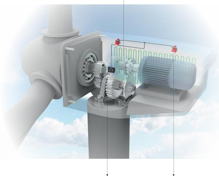
**2- Control unit** analyses the incoming signal in 10 milliseconds and activates the extinguisher tube. Simultaneously, it activates the alarm horn in the vehicle and warns the user by light-voice warning system on the panel.
