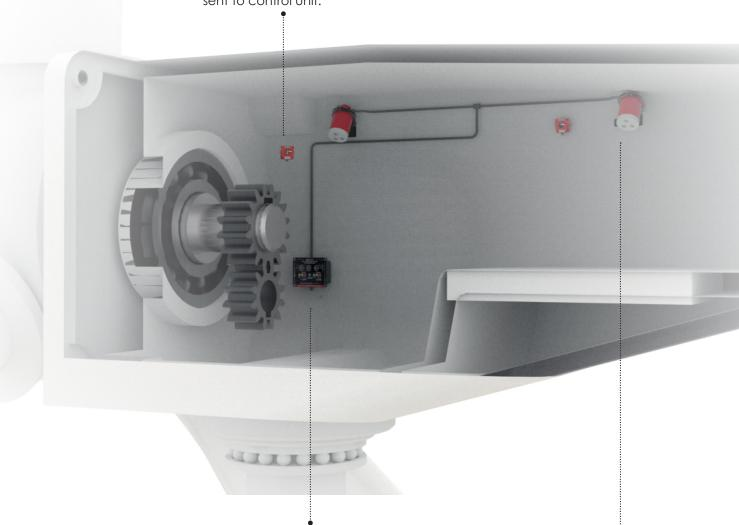
**2- Control unit** analyses the incoming signal in 10 milliseconds and activates the extinguisher tube. Simultaneously, it activates the alarm horn in the vehicle and warns the user by light-voice warning system on the panel.
