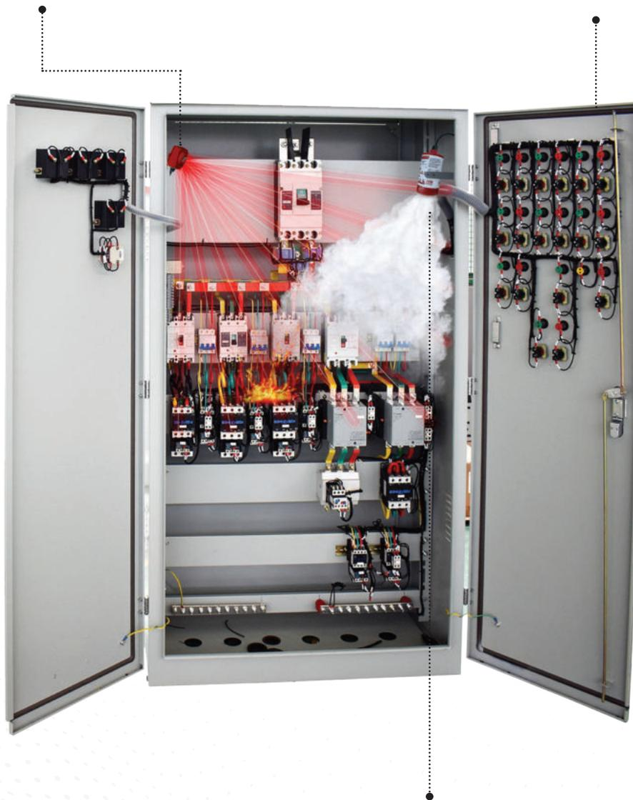
3- **The extinguisher tube** is activated with the help of the pyrotechnic trigger it has and extinguishing agents are released. The solid NRE-CM agent within the cylinder spreads homogenously and extinguishes the fire within five seconds.
