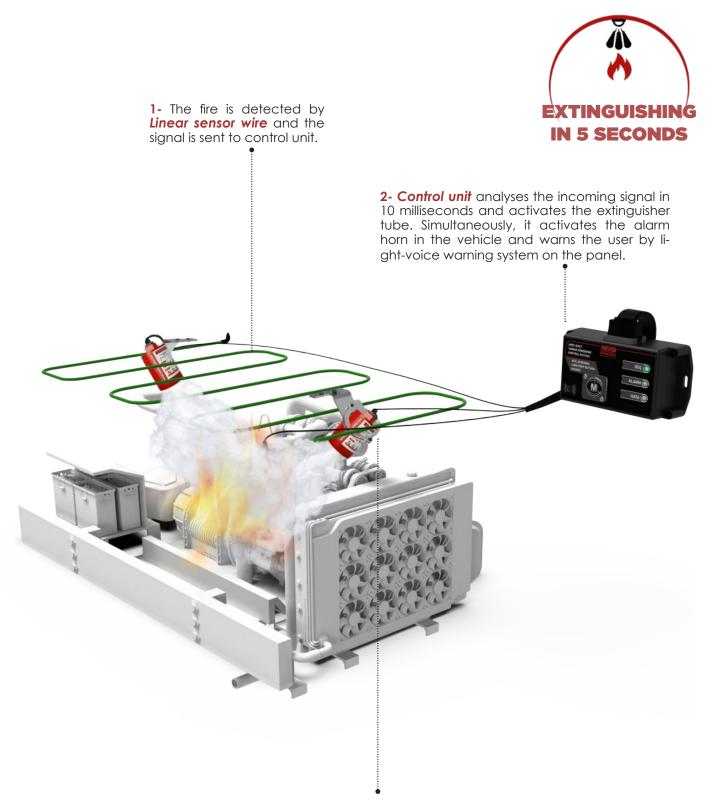
**3- The extinguisher tube** is activated with the help of the pyrotechnic trigger it has and extinguishing agents are released. The solid NRE-CM agent within the cylinder spreads homogenously and extinguishes
