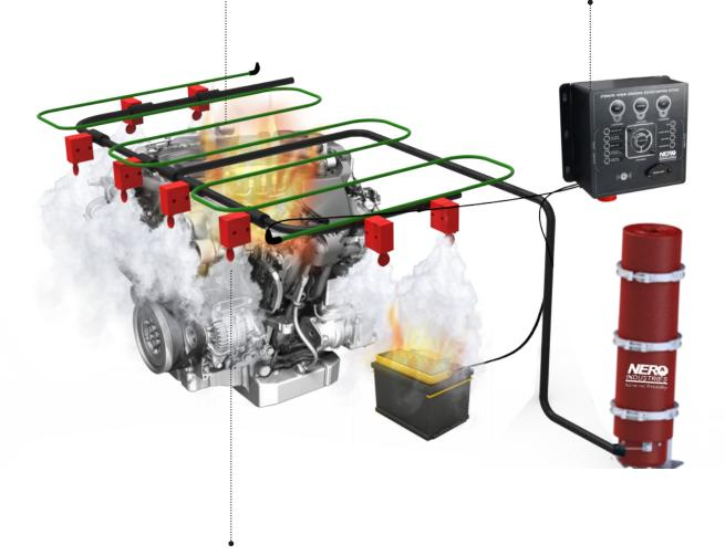
» 3- The extinguisher tube is activated with the help of the pyrotechnic trigger it has and extinguishing agents are released. Fire extinguisher tube delivers 2X FSS liquid extinguishing agent to nozzles within 2 seconds by the help of hydraulic lines.
