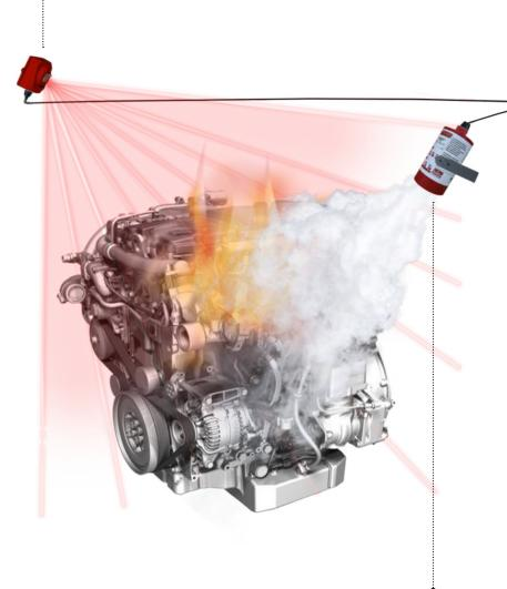
**3- The extinguisher tube** is activated with the help of the pyrotechnic trigger it has and extinguishing agents are released. The solid NRE-CM agent within the cylinder spreads homogenously and extinguishes the fire within five seconds.
