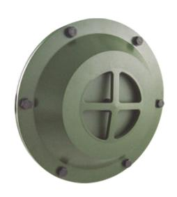
Blast valves are produced as relief valve on Positive Pressure CBRN Systems produced as per NATO AEP54 standards. The blast valves discharging CBRN system overpressure composed under proper conditions, are adjustable. Blast valves adjustable to requested pressure which have spring structure, can also be produced in special dimensions at user's request.
